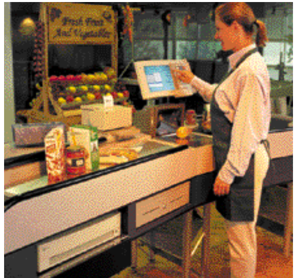
The NCR 7452, with the NCR DynaKey user interface, can be utilized in a modular configuration, as shown above, or an integrated configuration, as shown on the front.
